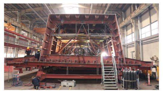
After fabrication and trial assembly completion of bridge decks were shipped to site by trucks.
