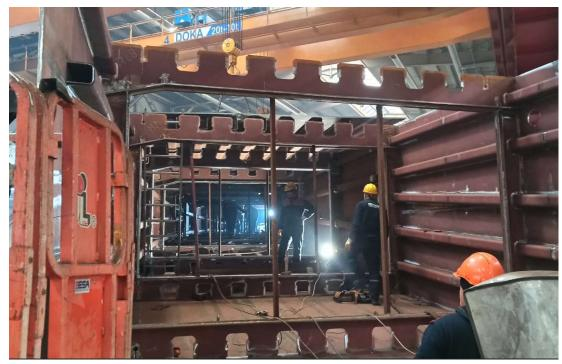
The bridge blocks were manufactured in seven modules in DOKA factory in Sakarya Hendek, and their painting was completed and shipped by trucks to the pre-assembly site in Belgrade, Serbia. The blocks vary between 6 meters and 24 meters.
